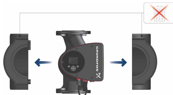
Fig. 3 Fitting insulating shells to the pump
