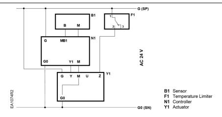
Figure 13. Connecting Terminals.
