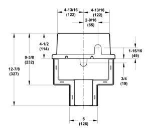
Figure 16. Dimensions of 599-10071 Weather Shield in Inches (Millimeters).
