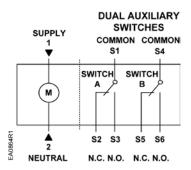
Figure 24. GCA12x, 2-Position Control.
