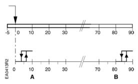
Actuator rotary range with the shaft adapter mounted at position "0".
