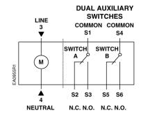
Figure 26. GCA22x, 2-Position Control.
