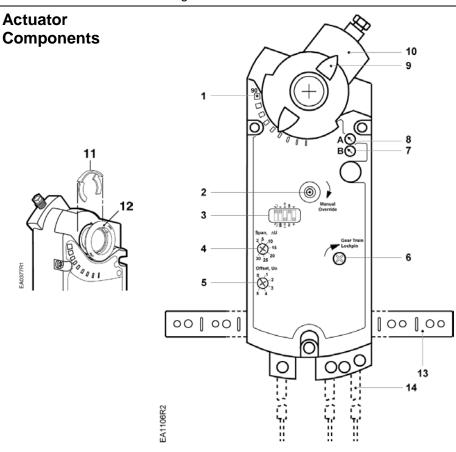
Figure 1. Modulating GCA Actuator.
