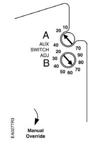
Figure 16. Dual Auxiliary Switch Dials.
