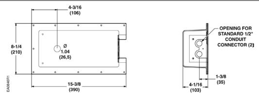
Figure 29. Dimensions of the ASK75.1U Weather Shield in Inches (Millimeters).
