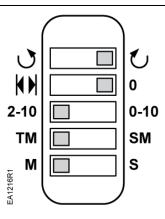
Figure 22. Tandem Application DIP Switch Settings.
