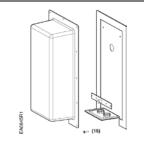
Figure 9. NEMA 3R Weather Shield.
