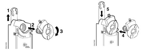
Figure 20. Mechanical Range Adjustment.
