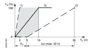
Ys Mechanical positioning range (100% = angle of rotation 90°)
