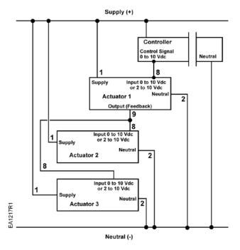
Figure 27. GCA15x.1x for Tandem Application (Master/Slave).
