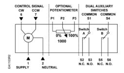
Figure 25. GCA13x, Floating Control.
