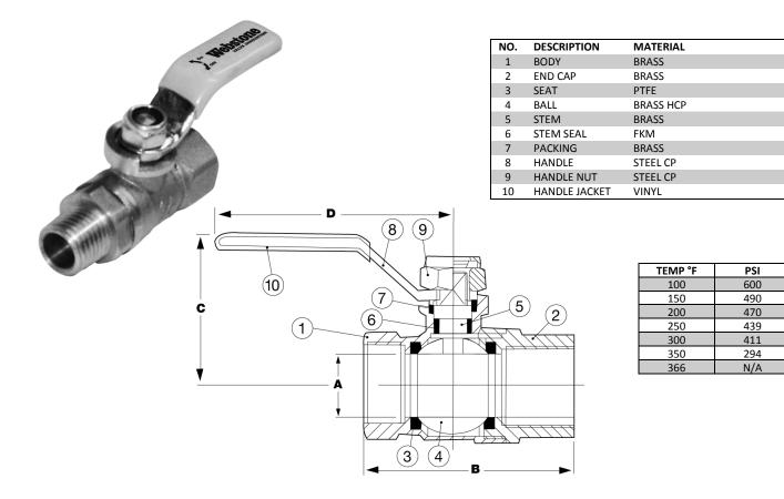
**Specifications:** Designed for commercial or industrial use with water, oil or gas. This approved Webstone valve is actuated by a blowout proof stem. Threaded ends comply with ANSI B1.20.1
