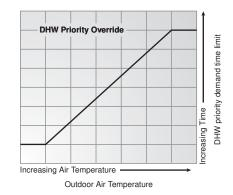
To provide external DHW priority, the boiler temperature space heating zones must be interlocked with the DHW Pmp / VIv contact. During DHW demands, the DHW Pmp / VIv contact must remove any power to all boiler temperature space heating zone valves or zone pumps.
