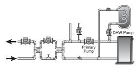
It is assumed that the DHW pump will provide adequate flow through the heat exchanger and the boiler.
