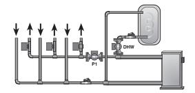
To prevent high temperature water from being introduced into the heating system, the boiler pump P1 must be turned off during a call for DHW. To do this, the DHW device must be a DHW pump (DIP switch = DHW Pump), DHW priority must be selected (DIP switch = DHW Priority), and BOIL MIN must be set to OFF.
