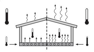
When a Taco Outdoor Sensor is connected to the Radiant Mixing Control (RMC), the RMC provides outdoor reset. When operating in the outdoor reset mode of operation, the installer must set the Outdoor Design Temperature and the Design Supply Temperature in order to establish the relationship between the outdoor temperature and the supply water temperature. This is known as setting the Heating Curve.
