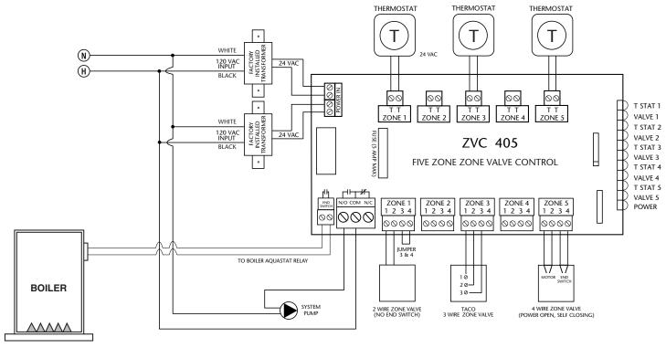
SYSTEM PUMP AND BOILER TURN ON WHEN ANY ZONE VALVE OPENS.
