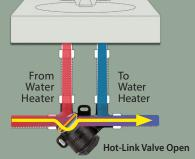
LEFT: No under-sink electricity needed. The Hot-Link circulator is mounted at the water heater.
